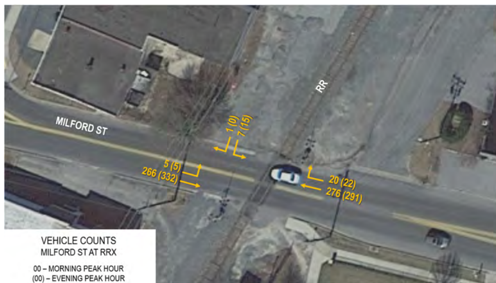
Figure 16: Vehicle Counts, Milford Street
